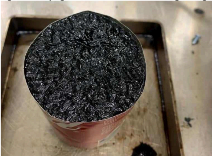
Figure 4 Clumping in the CR modified binder during the segregation test
