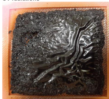
Figure 7 Conventional unmodified binder exposed to UV radiations
